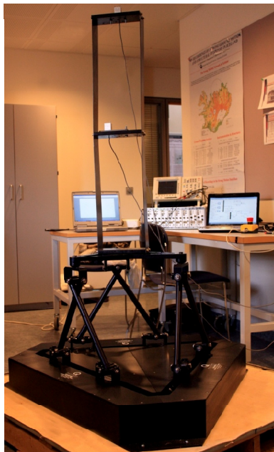
Figure 1 The Hexapod shake table supporting a two story structural frame model equipped with two accelerometers. In the background are control and monitoring devices.
