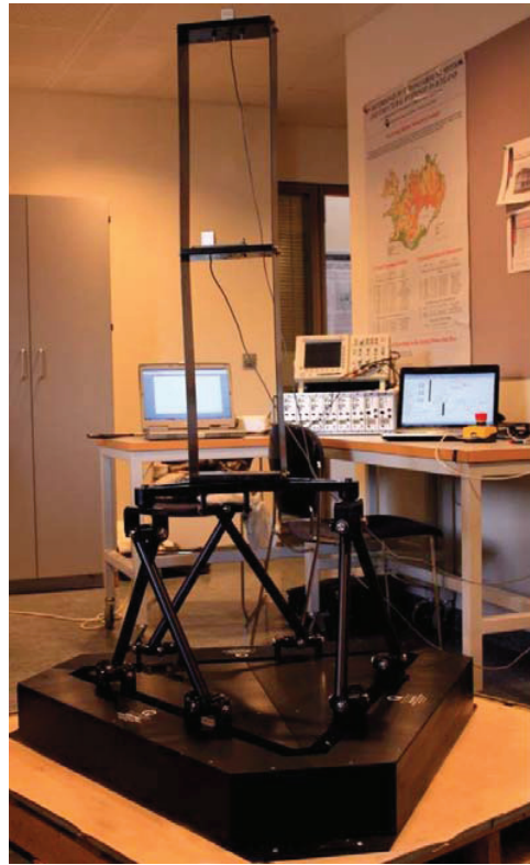
Fig. 1. The Hexapod shake table supporting a two story structural frame model equipped with accelerometric sensors. In the back-ground are control and monitoring devices.
